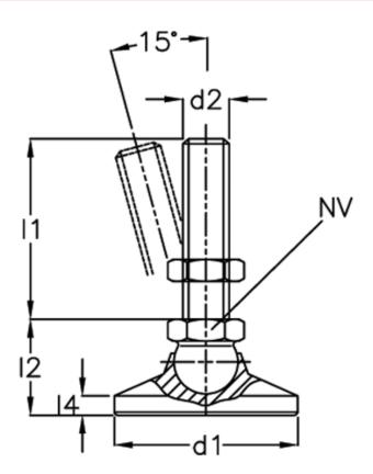
A/F = 15 d1 = 32 d2 = 10 l1 = 80 l2 = l4 = -Static load (N) = 20 Weight in (g) = 122
